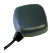
The WS3917 GPS antenna is a high value antenna with a wide voltage range, ideally suited to AVL and telematics platforms for vehicle-mounted use. Using internal magnets or screw mount holes, the antenna can be installed almost anywhere on a vehicle allowing great flexibility. The WS3917 antenna features a high gain (28 dB) low noise amplifier and a SAW filter. With a wide range of connectors and 2.7 to 5 volt operation, the antenna can be used with almost any GPS system available.
